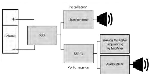
Figure 1: Sonomatter setup diagram for Installation and Performance.
