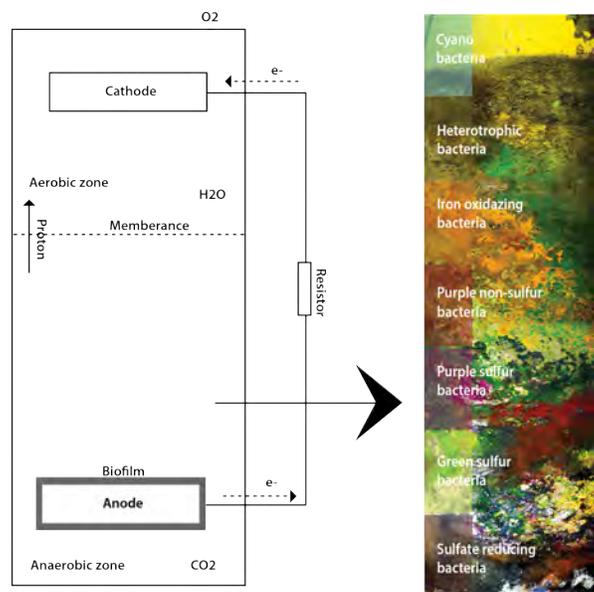
Figure 2: A MFC design and bacteria layers in Wino-gradsky Columns.
